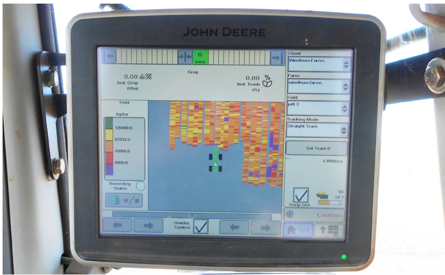
RiteYield integrated with John Deere 2630 displaying yield data in real time. Yield data are stored and displayed on the 2630 and may be transferred wirelessly using John Deere technology. The RiteYield console stores a data back-up in a common file format in internal memory for security and diagnostics purposes. Data can be copied at any time to the ruggedized USB flash drive.
