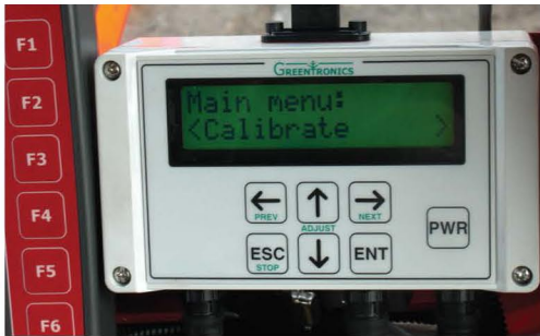
Controller with special rugged USB flash drive, sealed keypad and bright display to show harvest data and to navigate the menu system.
