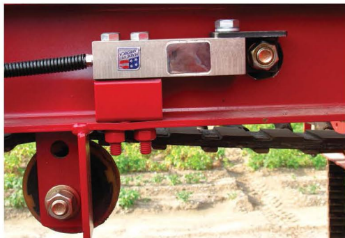
RiteYield system installed on Spudnik 3-row potato harvester, Alliston, ON, Canada
